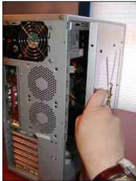
Figure 16: Removing the computer case cover
