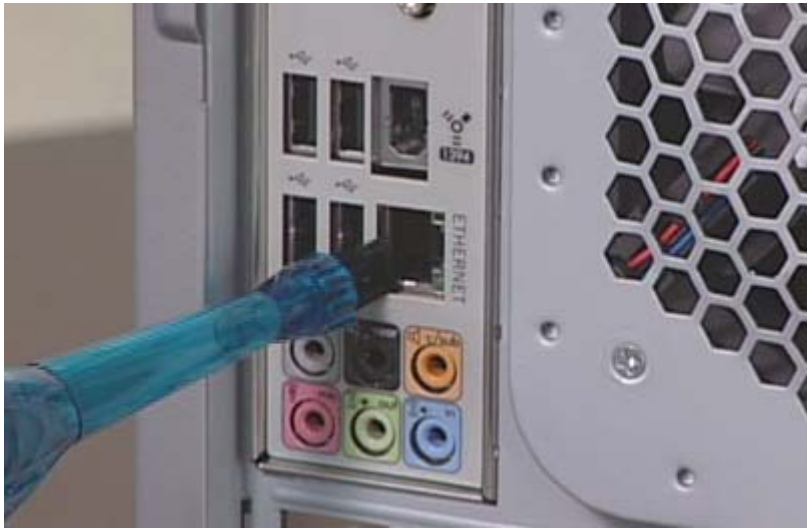
Figure 49: Various ports at the back of your computer
