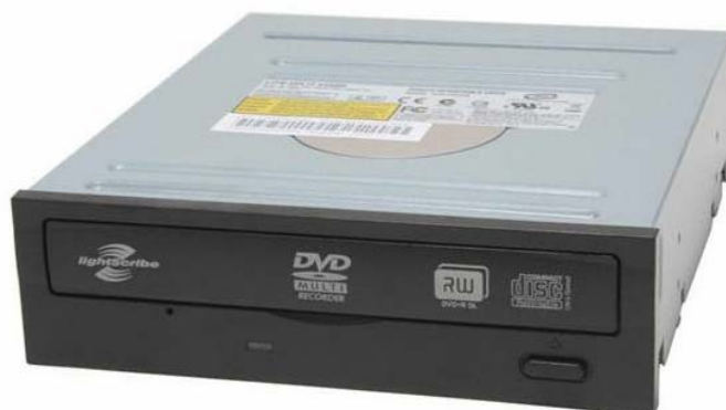
Figure 8: A typical DVD writer for a desktop computer
