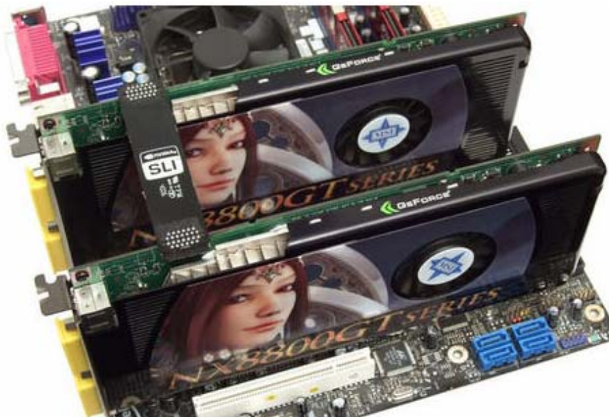
Figure 50: Dual nVidia video cards running in SLI configuration
