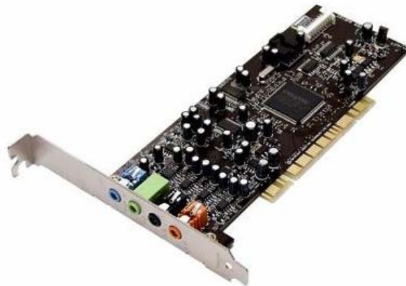
Figure 9: A typical sound card you find in a desktop computer
