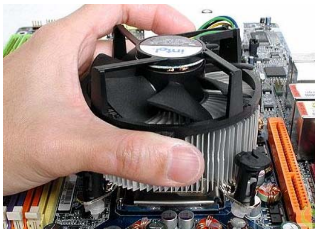
Figure 19: Installing the heatsink
