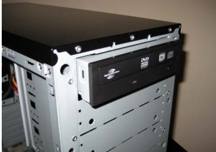
Figure 28: Load the DVD drive from the front of the computer case
